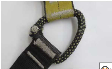
• Damaged attachment point
