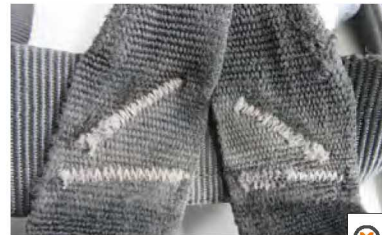
• Damaged safety stitching
