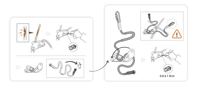
GRILLON replacement ropes, 2018 models up to 5 meters, are compatible with GRILLON models from January 2010 to May 2018, but this combination is not certified. Explanation:
