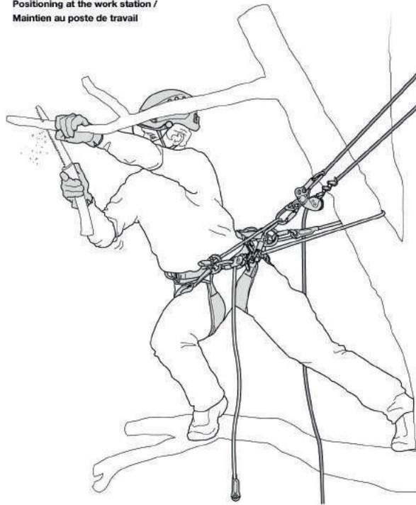
8c. Example of auxiliary attachment hole usage /
