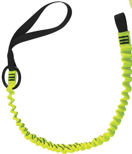
The RTLE3 is an elasticated tool lanyard with a choke loop for tool attachment and an 'O' ring for retention of a tool. It is suitable for tools up to 5kg in weight.
